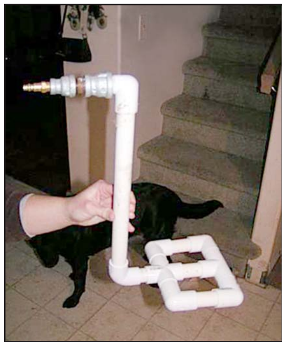
This is a homemade unit to clean eggs with water and bubbles. The unit is made with three-quarter-inch PVC pipe and drilled with a 3/32-inch bit. Photo by Mike Geubert.
