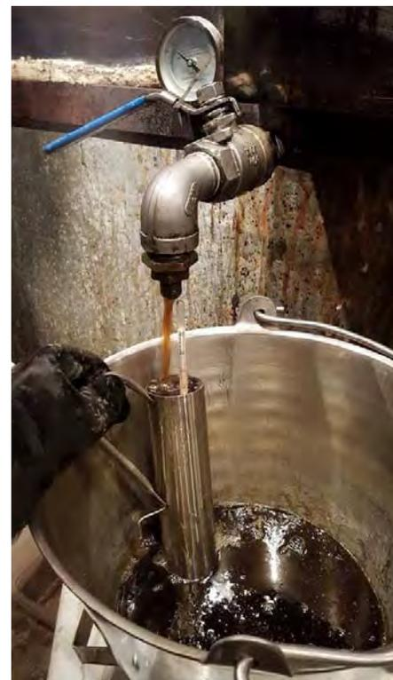
**Syrup Hydrometer:** Syrup hydrometers, like the one shown here, are what is required for measuring the higher percentage of sugar found in maple syrup. **Sap hydrometers:** Sap hydrometers are useful in determining which trees have sweeter sap and for calculating how many gallons of sap it will take to make one gallon of syrup according to Jones Rule of 86. Photo: Josh Penick, Hijinks Farm (NH)
