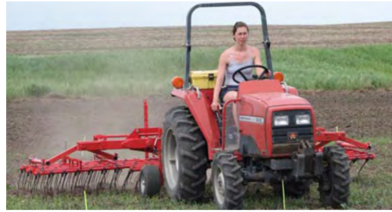
Harrows and non-selective tines weeding wild oats in tame oats. Photos: P. Shirliffe, University of Saskatchewan, Department of Plant Sciences
