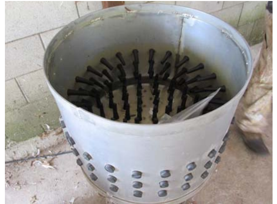
Feathers are removed by the abrasive action of rubber fingers in this tub-style picker. Photo: NCAT
