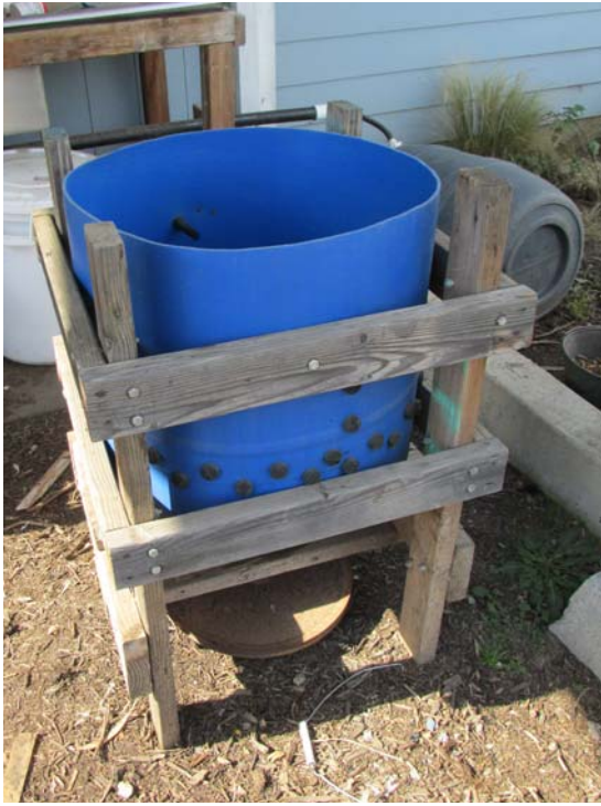
Pickers can be constructed from a plastic barrel, rubber fingers, and a small motor. Photo: NCAT
