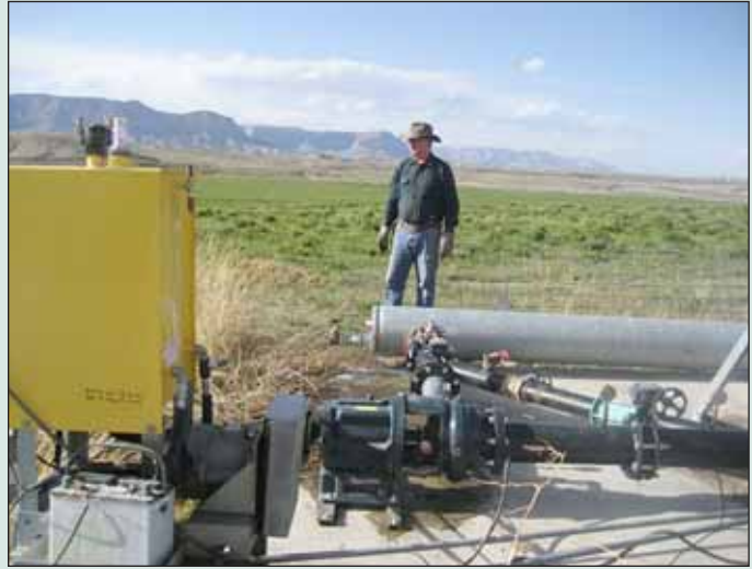
Roger Barton has eliminated all irrigation fuel costs by integrating a hydro turbine into his existing center pivot. Photo: Courtesy of Roger Barton
