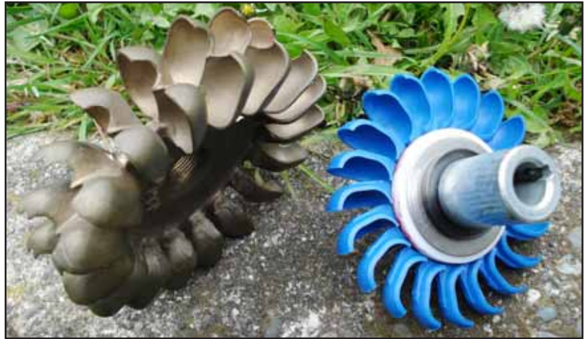
At left is a 4-inch pitch diameter Pelton wheel, and at right is a 3.24-inch pitch diameter Turgo wheel. Such wheel designs are common in micro-hydro systems. Photo: Leif Kindberg, NCAT
