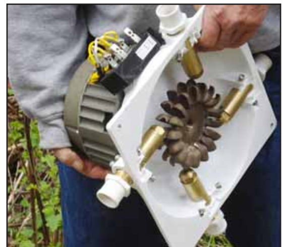
A custom-built four-nozzle hydro turbine with a bronze Pelton wheel and a brushless permanent magnet alternator. Photo: Leif Kindberg, NCAT
